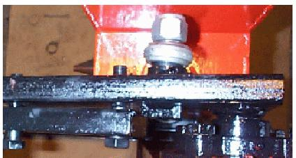
The red hand grip is welded to the shaft off-centre. There is a good reason for this so be careful in which direction the "long" side of the handle points. If you are standing facing the hopper, the
