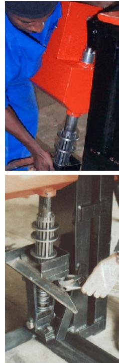
There is a rectangular hole machined into the side of the cylinder. This hole is open when the piston is up allowing seeds to enter the press. The bottom of this rectangular hole should be aligned with the bottom surface of the Hopper. This makes it easier to brush the last of the seed into the hole.
