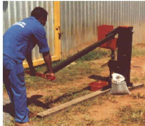
The second plank goes approximately under the path traveled by the handle. That is, the press stands on the centre of the plank so that one half is on the left of the hopper, the other half is on the right. When the handle is pushed down, it tries to pull the press over, and this pull is resisted by the plank which is resting against the ground. When the handle is thrown over to the other side, it presses against the other half of the plank.
