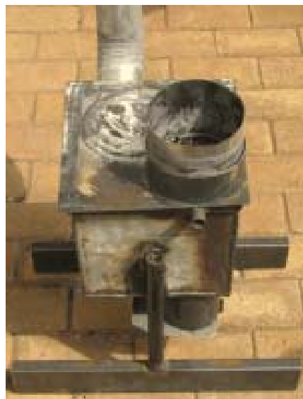
Figure 17: 16 mm tube added under the grate
