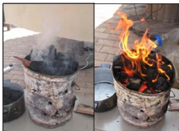
Figure 3: Conventional mbaulta: (a) Just starting to light emitting semi volatile organic smoke; (b) Well lit coal after ~30 minutes
