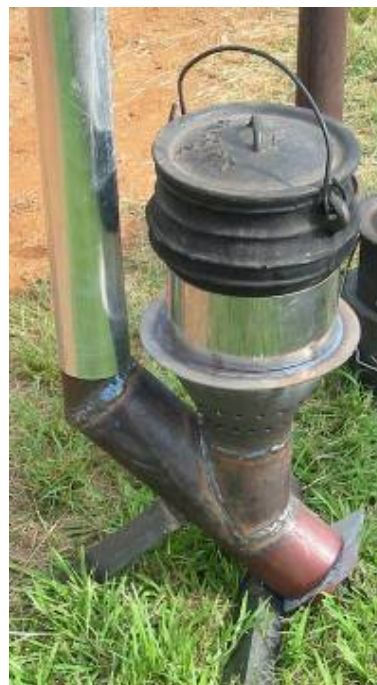
Figure 6: Single pot downdraft stove with air pre-heater and pot in place
