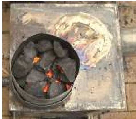
Figure 16: SeTAR Mk II BLDD coal stove with 125 mm diameter burner
