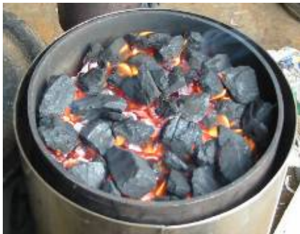
Figure 7: Partially pyrolysed coal in a double tube fuel hopper
