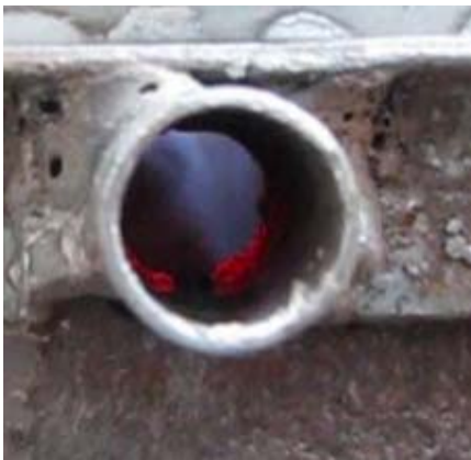
Figure 19: Combustion after pyrolysis is done
