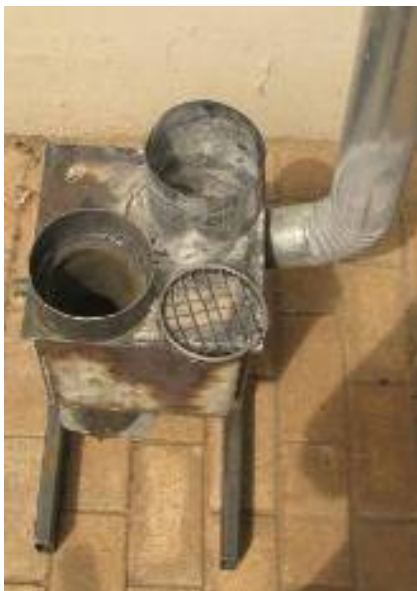
Figure 15: Combustor parts of the SeTAR Mk I BLDD coal stove
