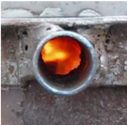
Figure 18: Combustion while pyrolysing in a SeTAR BLDD stove
